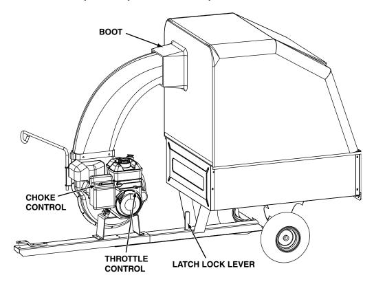
**LATCH LOCK LEVER** Locks the cart bed down to the tongue. Releases to allow cart to be tipped back for dumping.
